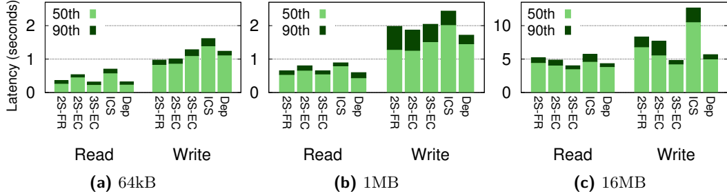
Figure 3 Median and 90-percentile latencies for read and write operations of register emulations.
