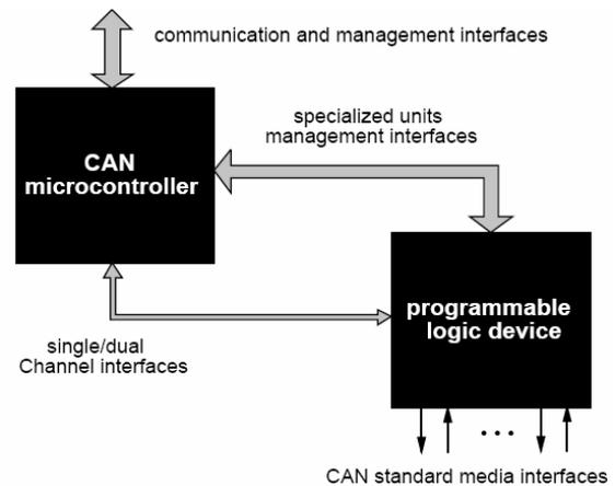
**Figure 2** CANELY Hardware Architecture
